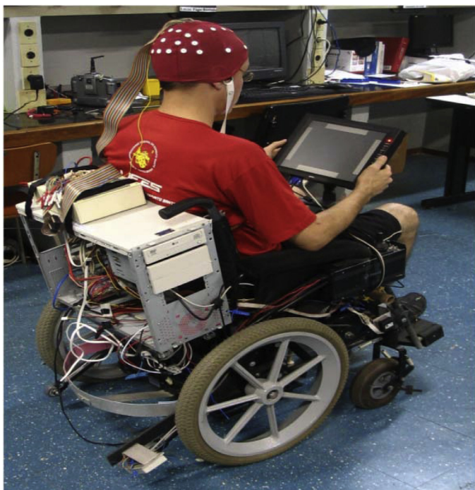
Fig. 5. EEG-based SSVEP command for wheelchair control adapted from [13].
